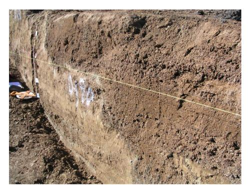
Figure 6. Channel fill next to the reddish paleosol that was in Soil Paleosol No. 2 (vertical tape) in the north wall of Trench FT-2.
