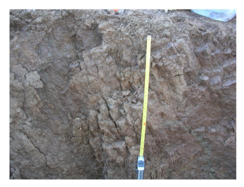
Figure 7. Tilted prismatic and angular blocky soil structure within the paleosol on the south wall of Trench FT-2 across from Soil Profile No. 3. The tilting is a result of soil creep that occurred when an active channel existed immediately to the east.
