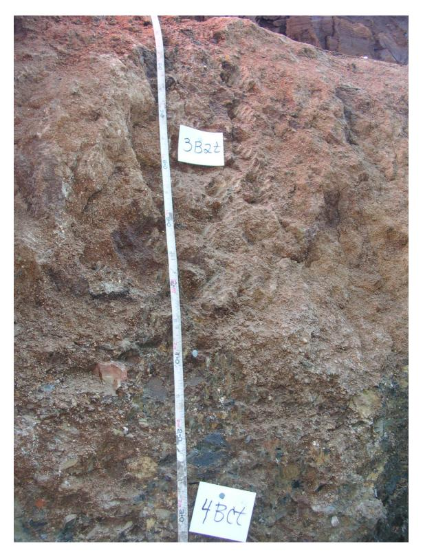
Figure 3. Bt/BCt contact at 210 cm in Soil Profile No. 1. Subtracting the fill, the actual depth would be 196 cm, with the Bt horizon being 175 cm thick.
