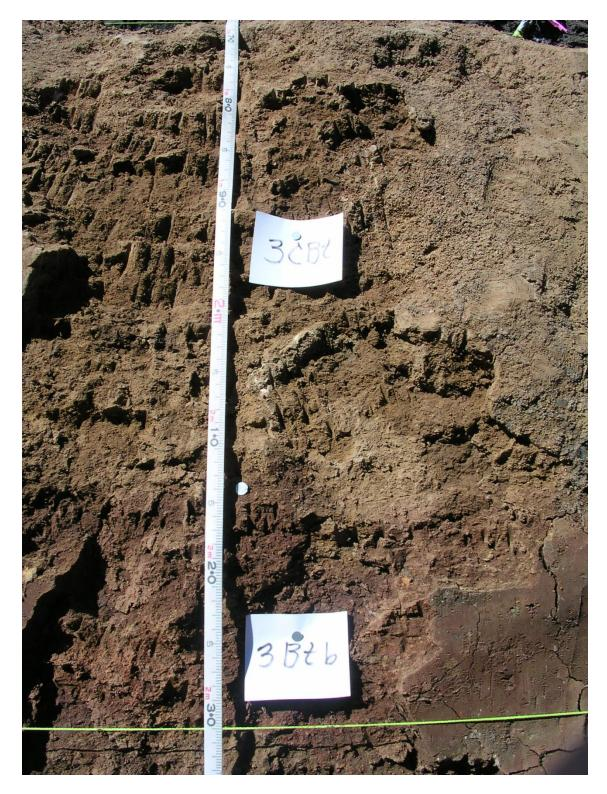
Figure 5. A reddish moderately well developed paleosol (horizon 3Btb) exists beneath the 214cm depth in Soil Profile No. 2 at Station 0 + 85 in Trench FT-2 west of the West Beverly Hills Lineament, which lies east of Beverly Hills High School. View N.
