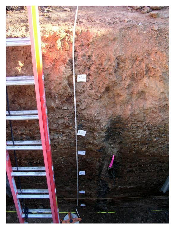
Figure 2. Lower portion of Soil Profile No. 1 at Station 0 + 43 in the south wall of Trench FT-1 west of the West Beverly Hills Lineament, which lies east of Beverly Hills High School. Clay film development reaches over 440 cm in this profile.
